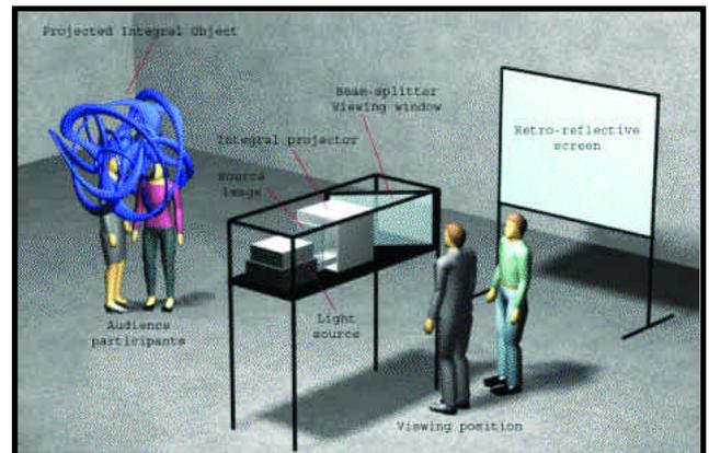
Fig. 10. CAD simulation of the cybersculpture installation
