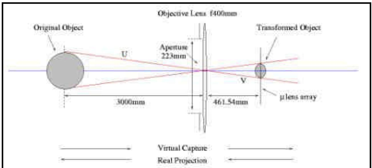
Fig. 9. Objective/projection lens parameters
